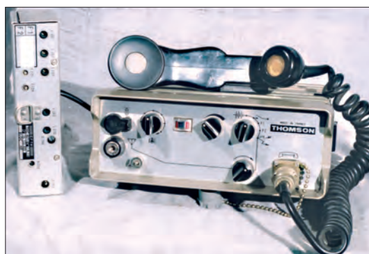
Fig. 3. The Thomson THC471 transceiver with optional plug-in frequency unit on the left. Note the very simple controls (see text).
