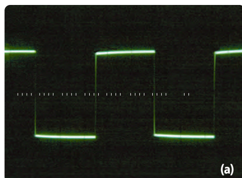
Fig. 3: Oscillogram (a) shows a squarewave taken directly from the output of a low distortion sinewave/squarewave oscillator. With the sweep control set to 10μs/div, a single cycle takes about 54μs, which means that the repetition frequency is close to 18.5kHz and the rise time about 0.1μs, but needing a faster sweep for a realistic assessment. Using the same sweep setting, oscillogram (b) takes about 35μs, putting the repetition frequency around 28kHz; but in this case the rise time is significantly longer at about 3μs.
