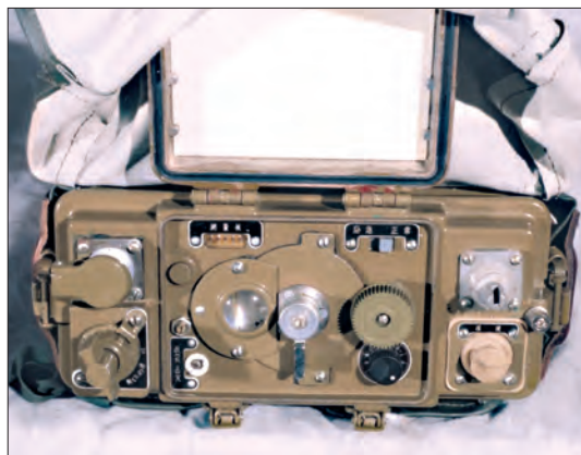
Fig. 1. The Chinese 884 v.h.f. set. The tuning window is just left of centre, the whip antenna fixes to the top right, with handset at the lower right (see text).
