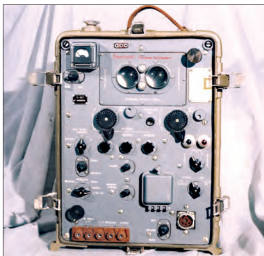
Fig. 4. The Russian P-407 v.h.f. set, the two glass windows are the tuning scales. The handset connects to the lower right with facilities for telephone line connection lower left (see text).
