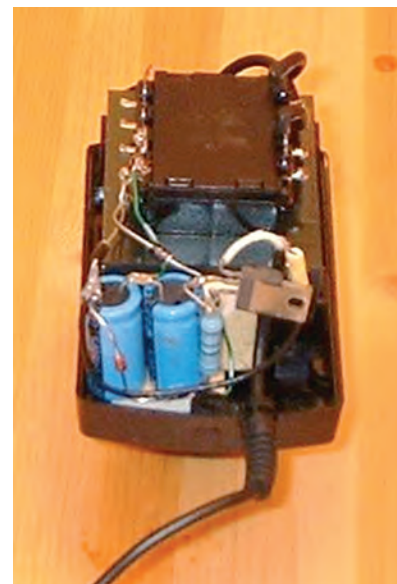
● Fig. 2 (above): As the relay's supply requirements are low, a simple 'wall-wart' supply is all that's needed.
