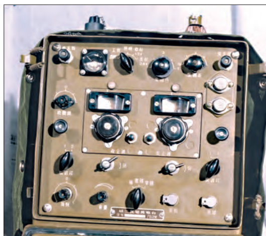
Fig. 2. The Chinese 73B h.f. manpack set. The receiver tuning is on the left, with the transmitter tuning on the right. Key and headphone sockets are on the lower right. The handset plugs in at the top of the set (see text).
